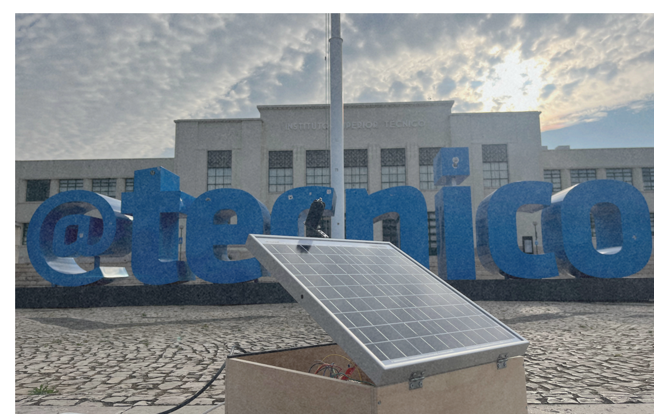
Final prototype: solar panel mounted for outdoor positioning tests
