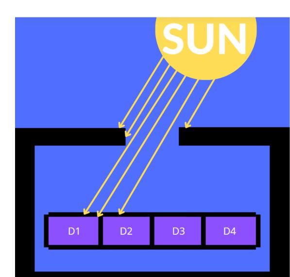
After conditioning and acquiring all photodiodes signals, the data is processed digitaly by an ESP-32 microcontroller which combines the information from all of the sensors on the satellite's faces and determines a "Sun Vector" which points to the deducted position of the Sun. This can later be communicated by the controller to the OnBoard Computer (OBC) which will use the information for attitude determination purposes.
