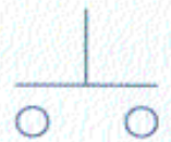
Normally open (NO) pushbutton
