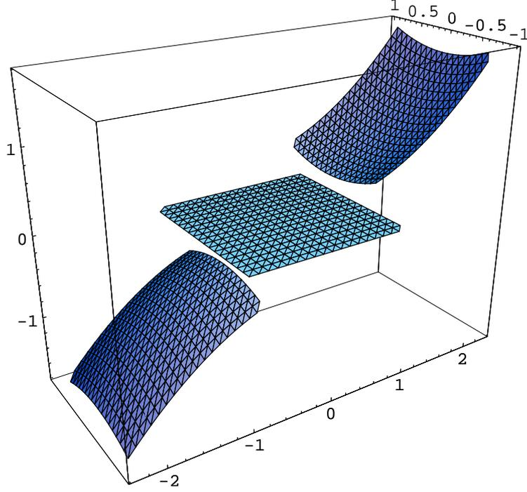
Figure 1: A mesh with 49 interior nodes, for each one of the three cracks.
