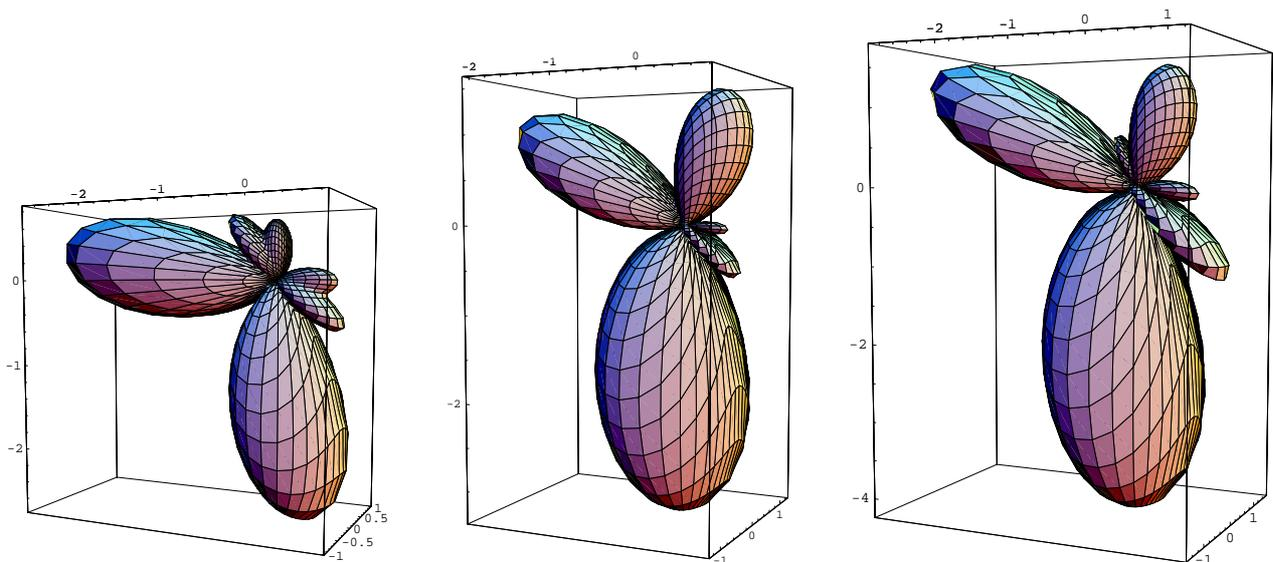
Figure 5: Far field modulus for an oblique plane crack (left) and with  $\alpha = 0.8, 1.0$ . (center and right)
