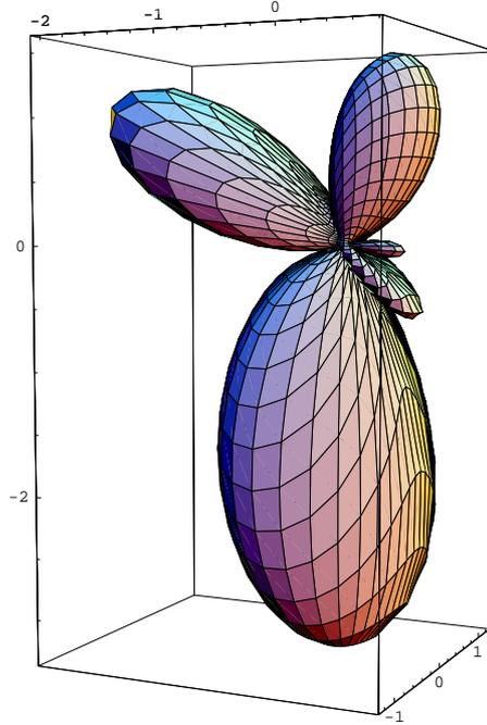
Figure 2: Modulus of the far field pattern generated by the 3 cracks with  $d = (0, 0, -1)$  and  $k = 2$ .
