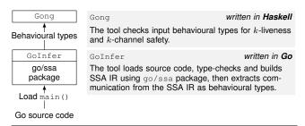
Figure 8. Workflow of our verification tool chain.
