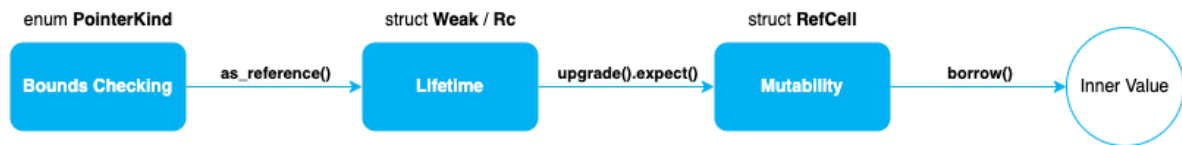
Figure 4.2: Steps for safely dereferencing a pointer in Rust using reference counting
