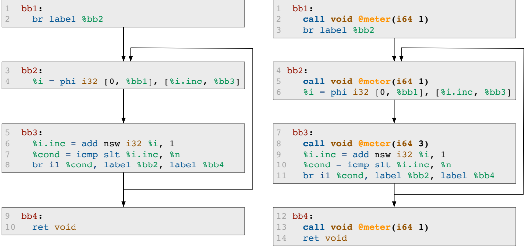
Fig. 19. Example of metering instrumentation as computed by the PB algorithm. For clarity, the metering is shown as a call to the @meter function which takes a single integer argument – a cost to update the budget of the program. We assume all LLVM instructions have unit cost.
