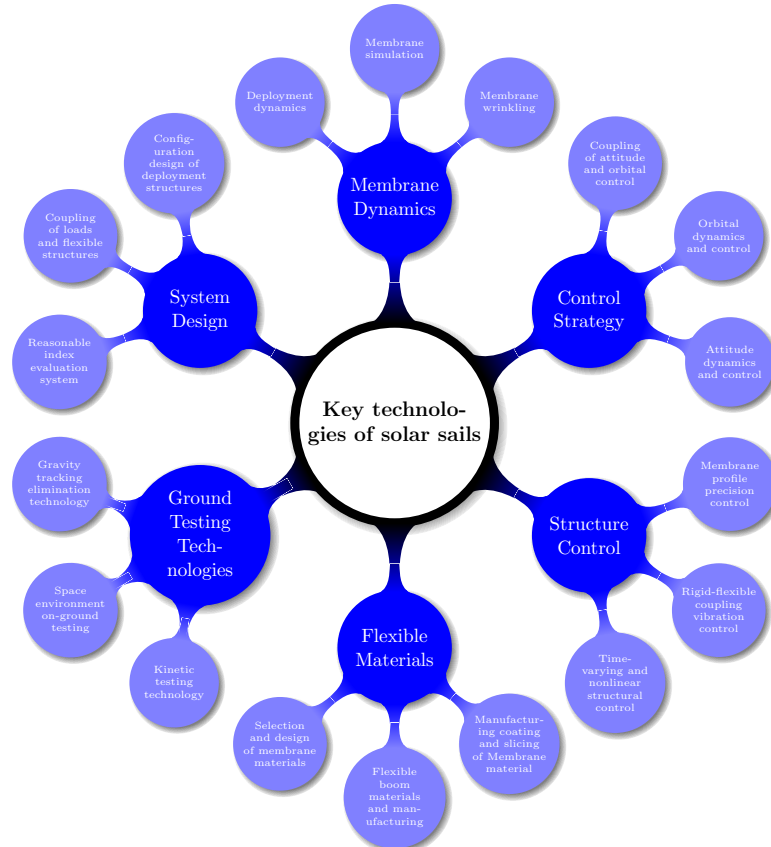
Figure 9: Key technologies of solar sails. (inspired by [18])
