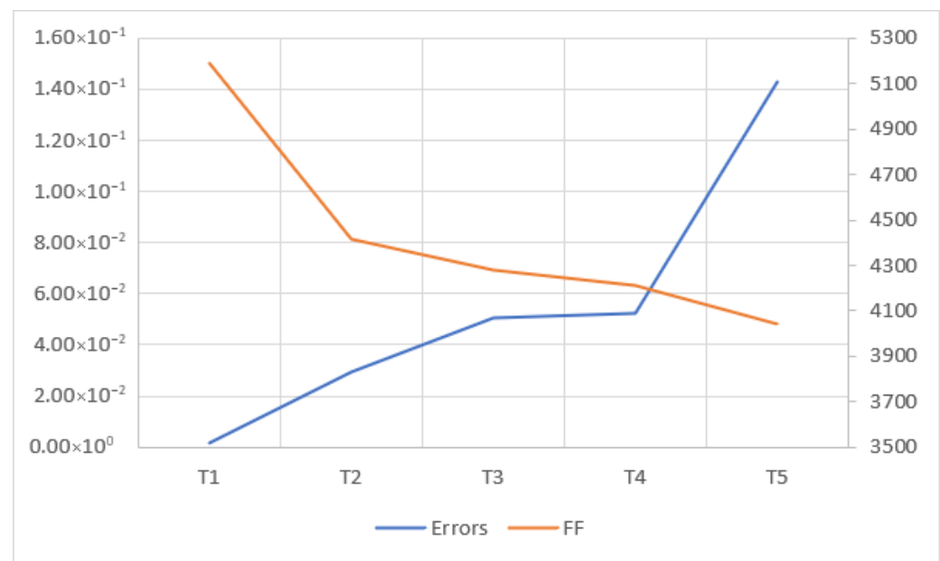
Figure 6. Graph of the tradeoff between the resources used (FFs) and errors of the output values (Maximum Absolute Value) when the word length decreases. The left axis corresponds to the errors. The right axis corresponds to the number of FFs.
