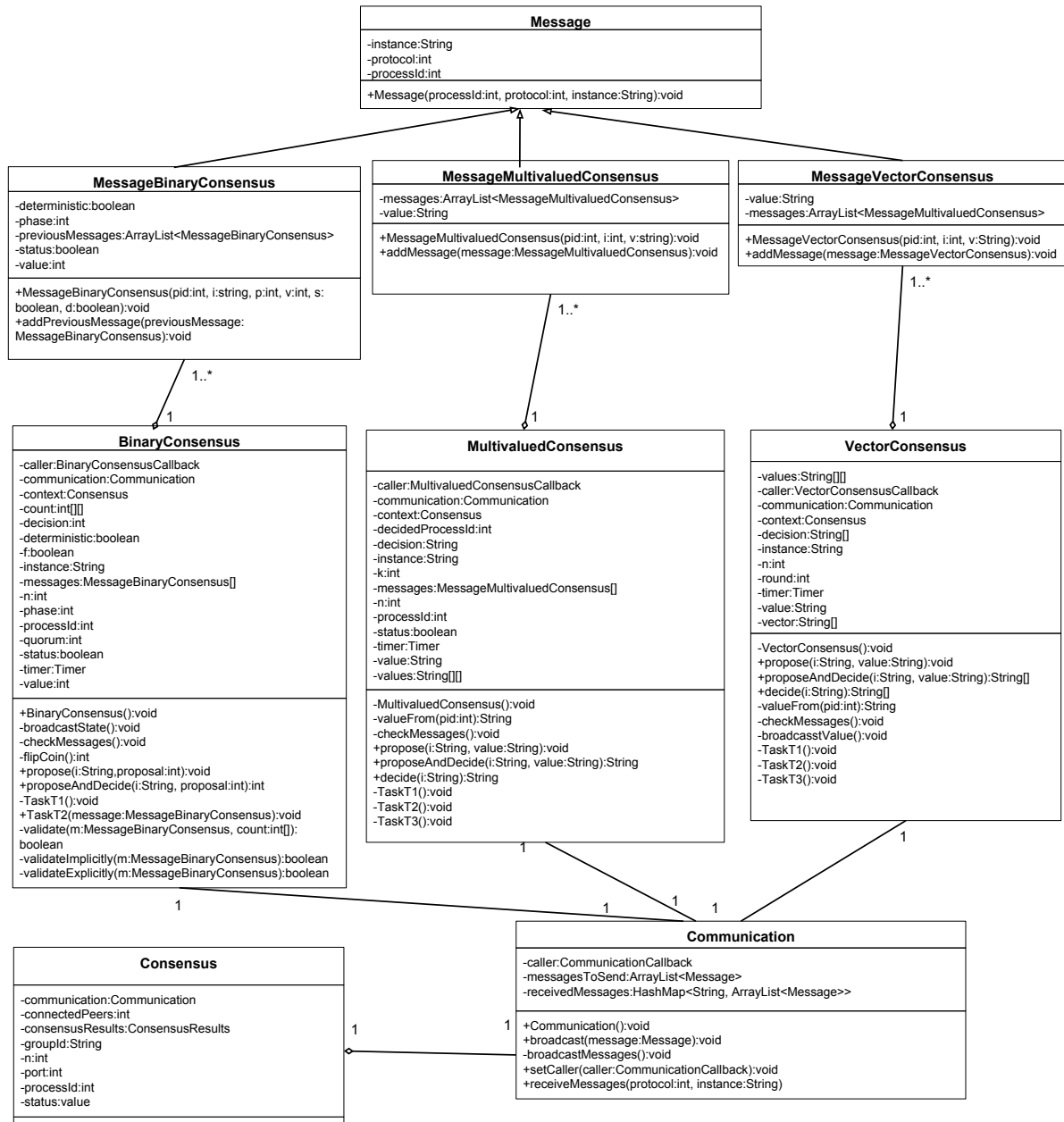
Figure 4.1: Class diagram of the android network library
