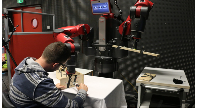
Fig. 1. Toolbox assembly with the help of Baxter robot. The robot hands over parts of the toolbox and hold them for the human coworker to screw them together.
