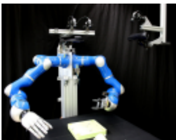
Figure 2. The experimental platform setup consisting of two KUKA lightweight arms, two DLR-HIT five-fingered hands, two Kinect cameras, four CMOS sensor cameras, and a motion capture system (the latter not visible in the picture).
