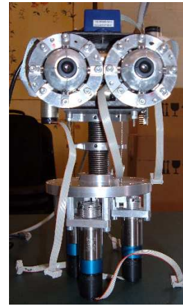
Fig. 4. Prototype of robot head with spring-based neck.
