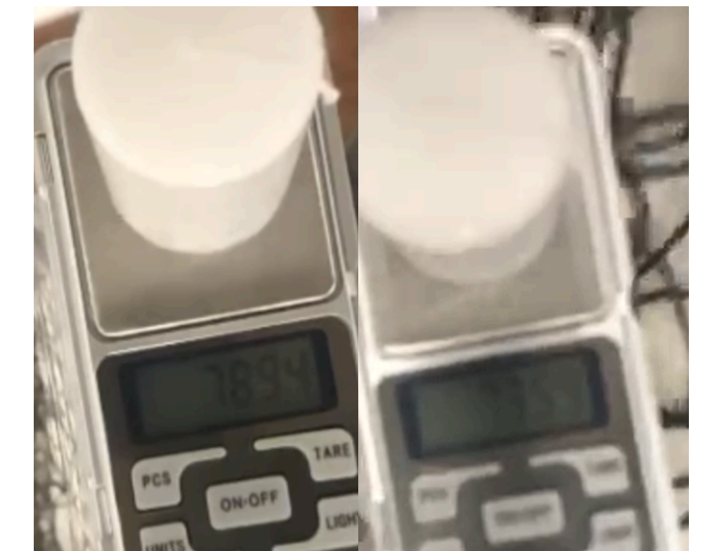
Experiment 2 - The scale read 78.94 grams at the beginning of the fall and 73.54 grams moments before landing.
