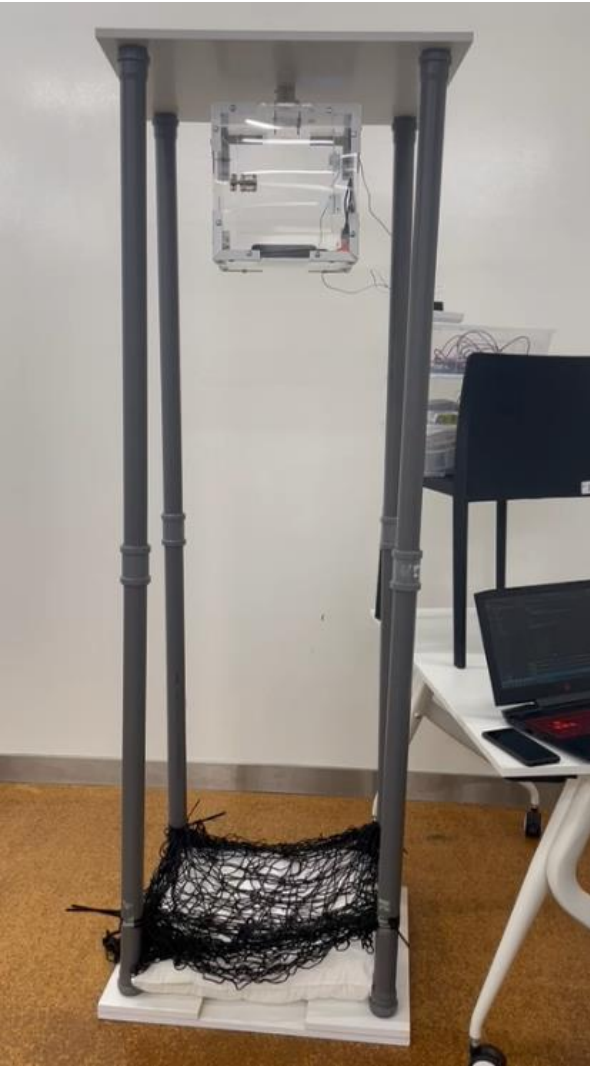
Full drop tower with Plexiglas box attached
