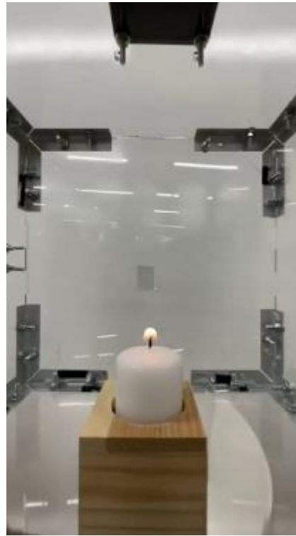
Side to side photos of an experiment with a candle (candle during free fall)
