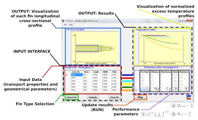
• The module solves the fin equation through a finite-volume approach.
