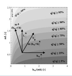
The adiabatic tip solution becomes a suitable approximation for an actual active tip for low values of  $q_{f,\mathrm{tip}}/q_f^c$  or high values of  $\mathbf{q}_{\mathbf{f}}^{\mathbf{a}}/\mathbf{q}_{\mathbf{f}}^c$ .
