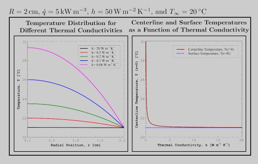
1 A surface energy balance applied to the cable cylindrical surface r = R can be considered to obtain the cable surface temperature,  $T_s$ , in alternative to the application of an energy balance to the overall cable – as considered in Equation (21). Note that the temperature gradient (dT/dr) in Equation (23) was evaluated with the temperature distribution provided by Equation (20).
