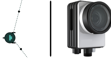
Figure 6.1: In bearing-only SLAM, the vehicle is equipped with sensors that are capable of measuring the relative direction to a landmark. For example, a single camera.
