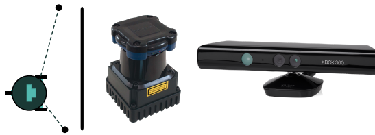
Figure 3.1: In range-and-bearing SLAM, the vehicle is equipped with sensors that are capable of measuring the position of a landmark relative to the vehicle. For example, a LIDAR in 2-D or an RGB-D camera for 3-D. In any of these cases, a feature detection/extraction tool has to be ran on the 2-D scans or the RGB images to obtain usable landmarks.
