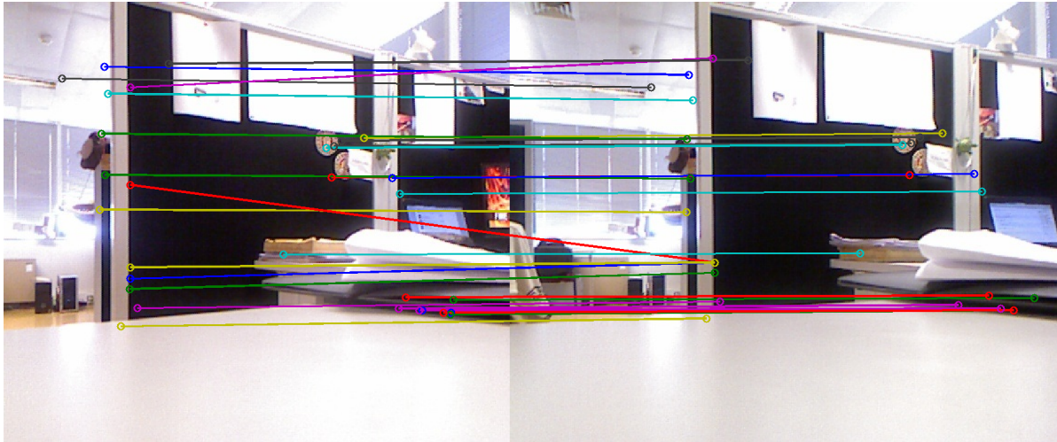
Figure 4.2: An example of the repeatability of features in two different images of the same scenery.
