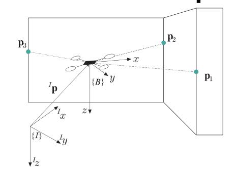
The **perception** of the environment by the vehicle is always **relative** to itself, due to the **sensors** involved. Exploring this idea, the algorithms we propose are designed in the space of the sensors. **Problems:**
