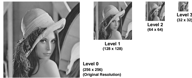
Figure 5. Application of a 4 layered decimation function to lenna test image.
