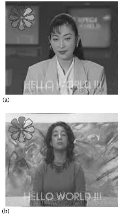
Fig. 26. Last frame (INTER type) of the first GOP (frame no. 8) of the Akyio (a) and Silent Voice (b) video sequences, processed using the open-loop DCT-domain transcoder with a GOP length M=8 ( Q=8 ). (a) PSNR = 33.07 dB and (b) PSNR = 31.52 dB.
