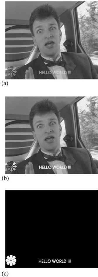
Fig. 3. Object insertion in the compressed DCT-domain using the CIF carphone video sequence and the transparency mask of (c): (a) \alpha = 0.5 ; (b) \alpha = 1 and (c) transparency mask, m(n_1, n_2) .
