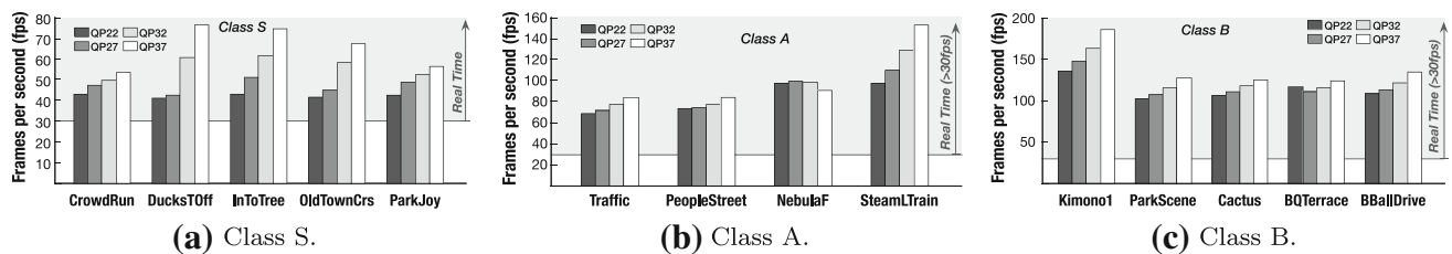
Fig. 15 Average frame rate obtained with the proposed GPU HEVC intra decoding modules on G780 GPU
