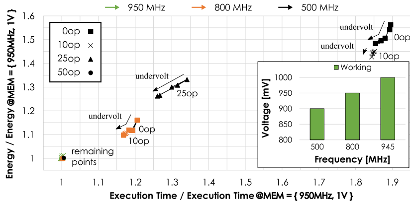
Fig. 2. DRAM DVFS in the VEGA 10 GPU: Normalized energy consumption, execution time and usable DRAM voltage for each frequency configuration.
