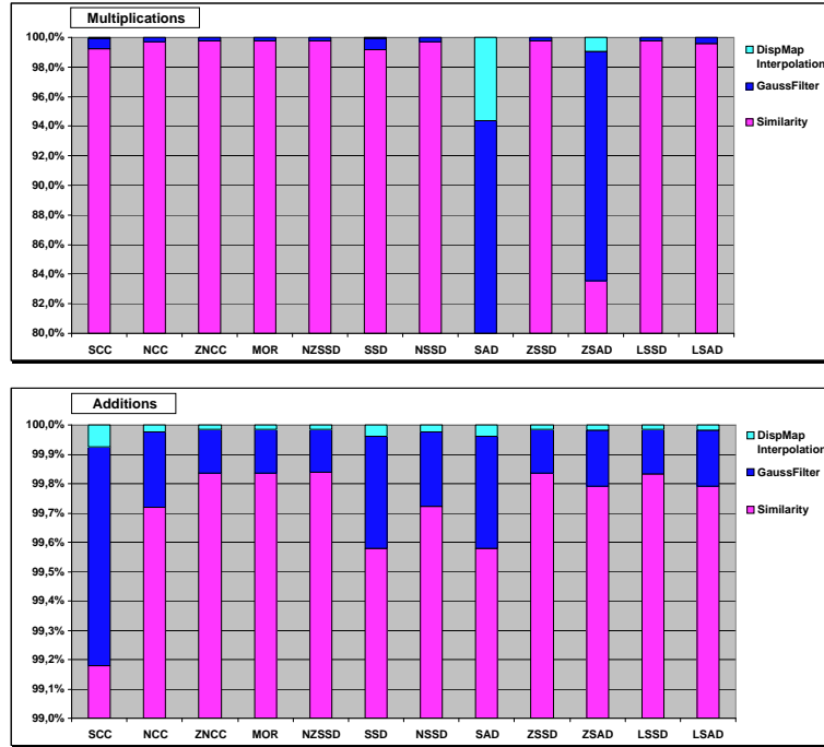
Fig. 18. Distribution of the multiply and add operations in the several stages of the system.
