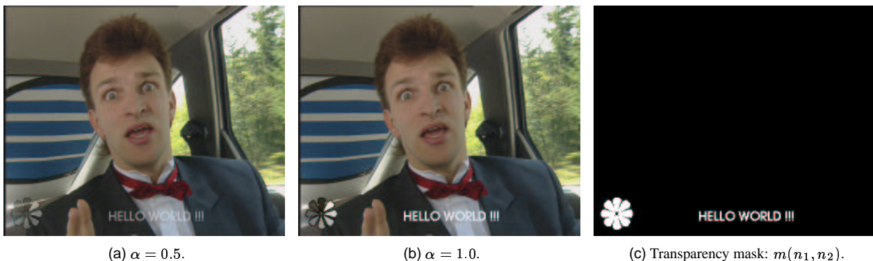
Figure 5. Logo insertion in the compressed domain using the carphone sequence and the transparency mask of fig 5(c).
