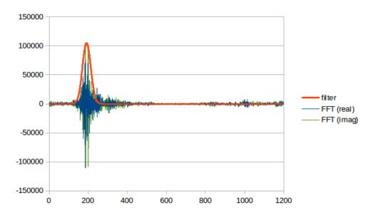
The idea is to apply a Gaussian filter around that point to keep only the main frequencies and throw away the rest.
