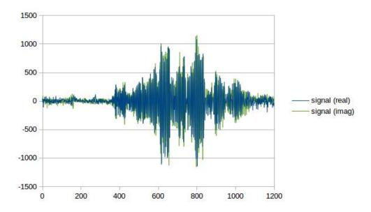
If we compute the FFT of this signal, we find that its main frequencies are located around the point 200 in the spectrum.
