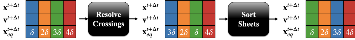
Figure A3. Illustration of changes in the array order after correcting for crossings. Colors represent the labels (array is omitted) and correspond to the sheets in figure A1 and figure A2. For simplicity, the values indicated in the \mathbf{x}_{eq}^{t+\Delta t} array represent the equilibrium position +\delta/2 . Once the corrections for crossings shown in figure A2 are applied, the final sheet positions, velocities, and equilibrium positions have changed. These arrays are then sorted with respect to the equilibrium positions, and not with respect to the sheet positions. This ensures that in the next time step, the crossing correction algorithm will be able to correct the crossings that were previously overlooked.
