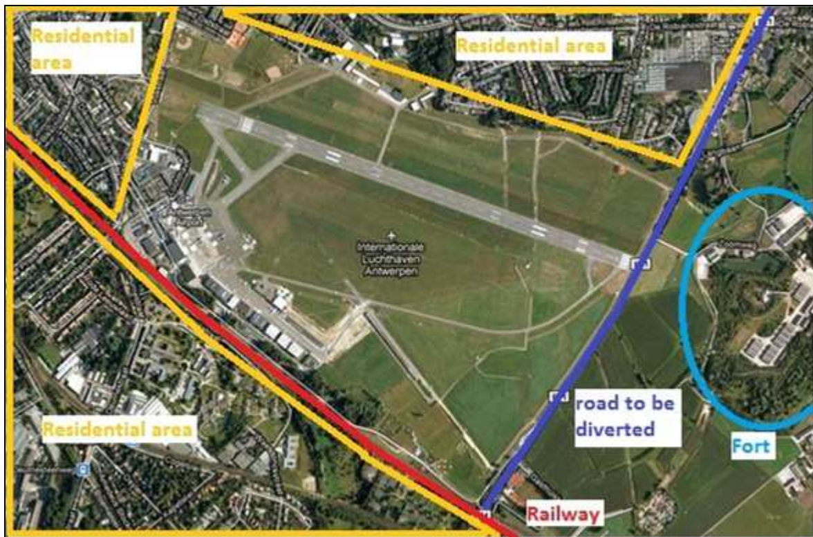
Figure 6.497: Picture of Antwerp Airport showing the restrictions for expansion
