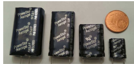
Fig. 14. Supercapacitors selected for the application (5 F, 3 F, 1 F and 0.1 F).
