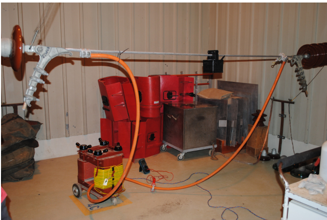
Fig. 2. Laboratory testing of a wireless sensor node (hanging on the line).
