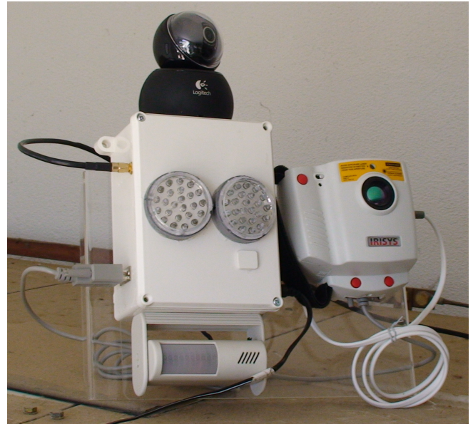
Fig. 4. Sensor node with web camera, light, motion detector and infra-red camera.
