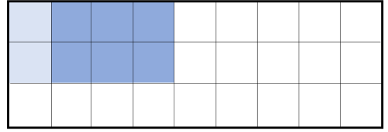
Fig. 2. An example of the kernel(3x2) and stride(1) on a 9x3 array
