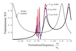
FIG. 2. (Color online) Amplitude of the transmission coefficient ( $S_{21}$  parameter) as a function of normalized frequency for the U-shaped ENZ transition depicted in Fig. 1 and different values of the losses  $\Gamma/\omega_p$ . The dashed line represents the transmission coefficient when the U-shaped transition is filled with air (empty channel).
