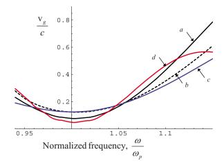
FIG. 8. (Color online) Group velocity as a function of the normalized frequency. The collision (damping) frequency is such that  $\Gamma/\omega_p$ =0.001, except for curve b where  $\Gamma/\omega_p$ =0.05. Curves a (solid black line) and b (dashed black line):  $a_{ch}$ =0.1a and L=1.0a. Curve c (blue line, dark gray in gray scale):  $a_{ch}$ =0.2a and L=1.0a. Curve d (red line, light gray in gray scale):  $a_{ch}$ =0.1a and L=2.0a.
