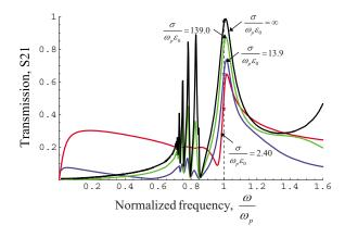
FIG. 7. (Color online) Amplitude of the transmission coefficient ( $S_{21}$  parameter) as a function of normalized frequency for a U-shaped ENZ channel and different values of the conductivity of the walls. The "star" symbols along the vertical line  $\omega = \omega_p$  represent the results computed using formula (8).
