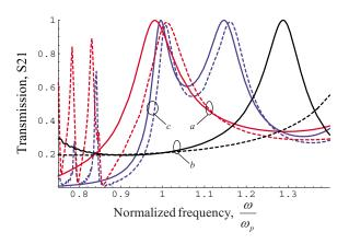
FIG. 9. (Color online)  $S_{21}$  parameter as a function of normalized frequency for an artificial plasma (solid lines) emulated using a 3D metallic waveguide and for the corresponding 2D setup of Fig. 1 (dashed lines). (a) U-shaped transition with L=1.0a. (b) 3D waveguide uniformly filled with  $\varepsilon_{d,r}=2.0$  (solid line) and the corresponding 2D setup with the narrow channel filled with air (dashed line). (c) Similar to (a) but with L=3.0a.
