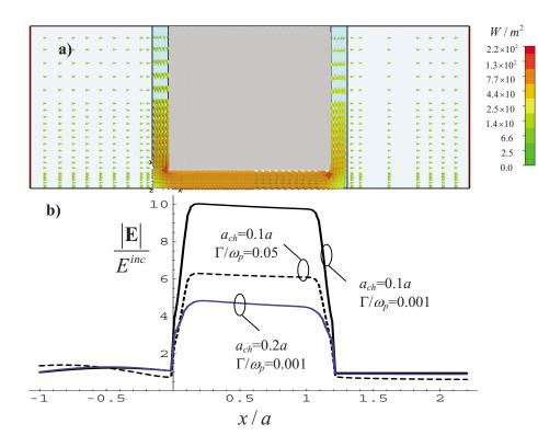
FIG. 5. (Color online) Panel (a): Real part of the Poynting vector for  $a_{ch}$ =0.1a and  $\Gamma/\omega_p$ =0.001. Panel (b): Electric field (normalized to the amplitude of the incoming wave) along the line y=0.5 $a_{ch}$  for different values of the loss parameter and of the channel height.
