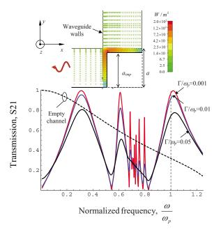
FIG. 3. (Color online) Upper panel: Real part of the Poynting vector lines in a waveguide with a 90° bend filled with a ENZ material at  $\omega = \omega_p$  and negligible losses. Lower panel: Amplitude of the transmission coefficient ( $S_{21}$  parameter) as a function of normalized frequency and different values of  $\Gamma/\omega_p$ . The dashed line represents the transmission coefficient when the 90° bend is filled with air (empty channel).
