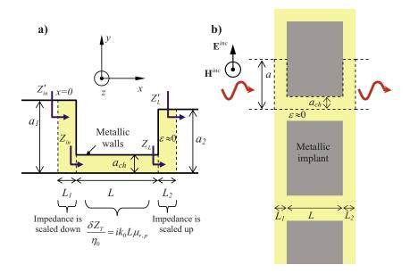
FIG. 4. (Color online) Panel (a): Illustration of the wave impedance transformations inside the U-shaped channel. Panel (b): A ENZ slab periodically loaded with metallic implants is illuminated by a plane wave that propagates along the normal direction.
