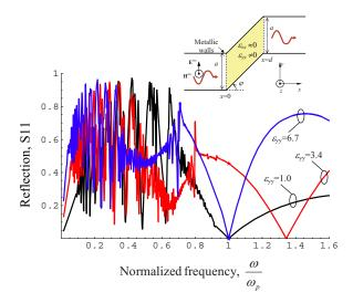
FIG. 12. (Color online) Reflection characteristic of a waveguide filled with a ENZ anisotropic material as a function of normalized frequency. The star symbols at  $\omega = \omega_p$  represent the theoretical values computed using Eq. (21). The distance between the upper and lower plates is uniform in the ENZ section. The inset represents the geometry of the structure.
