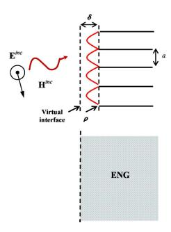
FIG. 4. (Color online) Virtual interface concept: A plane wave with polarization parallel to the metallic plates is scattered by the parallel plate metamaterial (upper panel) in the same way as it would be scattered by an equivalent ENG material (lower panel) with interface displaced a distance  $\delta$  from the physical interface.
