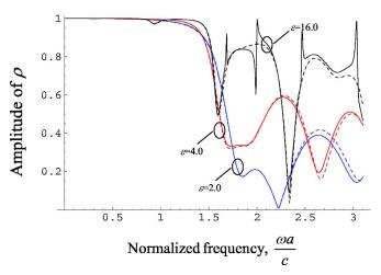
FIG. 9. (Color online) Amplitude of the reflection coefficient as a function of the normalized frequency for different DPS slabs with thickness  $d_1$ =1.0a. The effective thickness of the metamaterial slab is  $d_2$ =1.0a and the permittivity of the dielectric between the metallic plates is  $\varepsilon_{\rm diel}$ =4.0. Solid lines: Full wave numerical result. Dashed lines: Homogenization theory results taking into account the effect of virtual interfaces.
