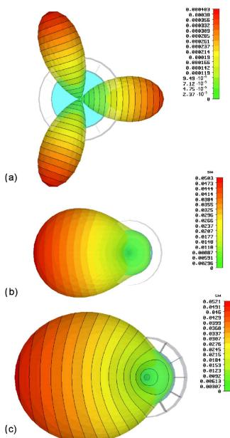
FIG. 20. (Color online) Far-field radiation patterns in the three cases of Fig. 18 [notice how in (a) the scale is different, and much lower, with respect to the other cases].
