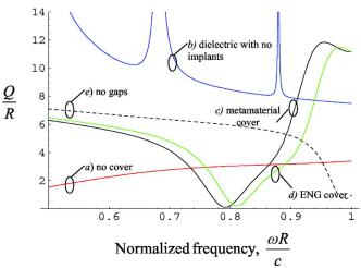
FIG. 17. (Color online) The effect of the virtual interface: Normalized scattering width as a function of the normalized frequency. (a) Cylindrical dielectric object with no cover. (b) Object covered with a dielectric shell with  $\varepsilon$ =38.8. (c) Object covered with metamaterial (dielectric shell+12 implants). (d) Ideal ENG cover following the Drude model (36). (e) Object covered with metamaterial with no gaps.
