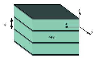
FIG. 1. (Color online) Geometry of the parallel-plate medium as a metamaterial: A periodic set of vanishingly thin metallic plates filled with a dielectric with permittivity  $\varepsilon_{\rm diel}$ .
