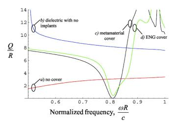
FIG. 14. (Color online) Normalized scattering width as a function of the normalized frequency. (a) Cylindrical dielectric object with permittivity  $\varepsilon=3$  and radius R, with no cover around it. (b) Object covered with dielectric shell with  $\varepsilon=35.4$ . (c) Object covered with metamaterial (dielectric shell+12 implants). (d) Ideal ENG cover following the Drude model (36).
