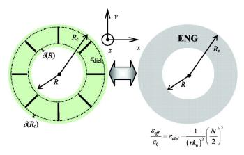
FIG. 12. (Color online) Equivalence between a cylindrical radial-plate metamaterial shell and an ideal ENG cylindrical shell. The analogy is valid as long as the electric field is parallel to the plates, following the results of Sec. II.
