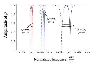
FIG. 10. (Color online) Amplitude of the reflection coefficient as a function of the normalized frequency when the metamaterial slabs are juxtaposed to different MNG slabs. Solid lines: Full wave numerical result. Dashed lines: Homogenization theory results taking into account the effect of virtual interfaces.
