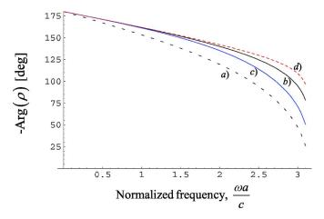
FIG. 5. (Color online) Phase of the reflection coefficient in a semi-infinite parallel plate medium for the angle of incidence  $\theta$ =45°. (a) Homogenization model without virtual interface. (b) Exact result. (c) Homogenization model with the virtual interface. (d) Homogenization model with the virtual interface calculated with a more accurate formula.
