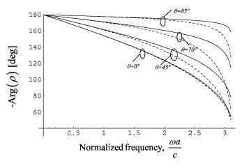
FIG. 6. Phase of the reflection coefficient for a semi-infinite parallel plate medium for incidence along  $\theta$ =0°, 45°, 70°, and 85°. Solid lines: Exact result. Dashed lines: Homogenization model with virtual interface (using  $\delta \approx 0.1a$ ).
