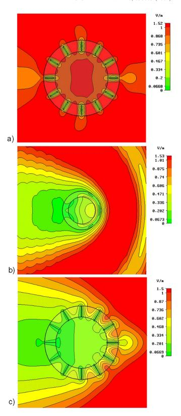
FIG. 18. (Color online) Electric field amplitude for the case of Fig. 14 at the frequency for which  $k_0R$ =0.8 in the three cases of (a) with cover designed as in Fig. 14, (b) with the same cover, but removing the metallic plates, and (c) again with the same cover, but with metallic plates extended also in the virtual interface.
