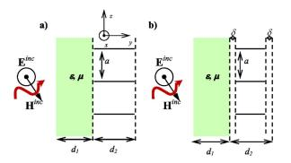
FIG. 2. (Color online) A magnetodielectric slab juxtaposed to metallic waveguides below cutoff. Panel (a): The plates are adjacent to the dielectric slab. Panel (b): Gaps of width  $\delta$  are placed at the interfaces between the plates and the dielectric and free space.
