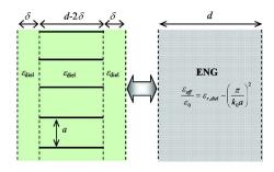
FIG. 7. (Color online) Equivalence between a metamaterial slab with proper virtual interfaces and an ENG medium.
