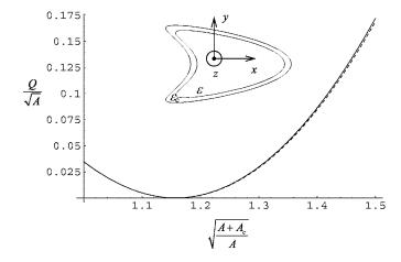
FIG. 11. Normalized scattering width Q for a kite-shaped cylindrical object (as depicted in the inset) as a function of the normalized radius of the plasmonic cover. The permittivity of the object is  $\varepsilon=3$  and the one of the cover is  $\varepsilon_c=-5$  at the design frequency. Solid line: Incident plane wave propagates along the x direction. Dashed line: Incident plane wave propagates along the y direction. The electric field is polarized along z.
