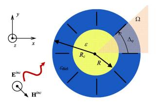
FIG. 13. (Color online) Geometry under analysis: A dielectric cylinder covered with a radial-plate metamaterial consisting of conducting implants embedded in a dielectric shell. The unit cell  $\Omega$  is shown.
