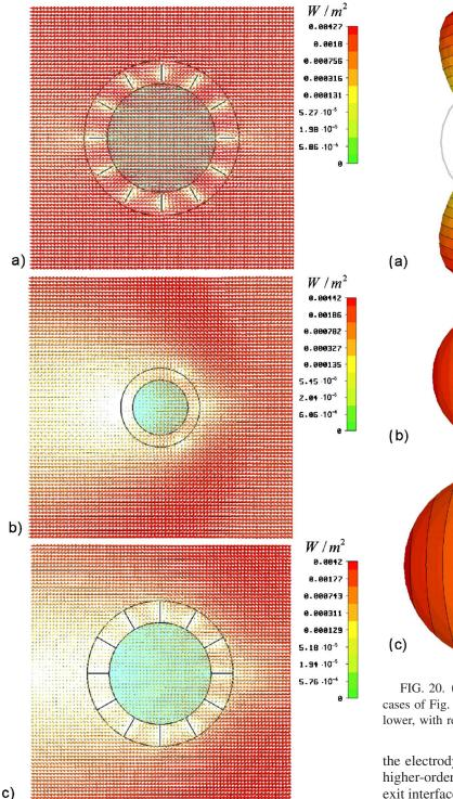
FIG. 19. (Color online) Power flow (real part of the Poynting vector) in the three cases of Fig. 18.
