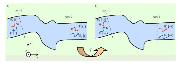
**Figure 1.** Illustration of the effect of the time-reversal operation in a time-domain scattering problem: (a) The incoming waves  $E_1^+$  and  $E_2^+$  are scattered by the junction and originate two outgoing waves  $E_1^-$  and  $E_2^-$ . (b) Time-reversed scenario where the roles of the incoming and outgoing waves are exchanged.
