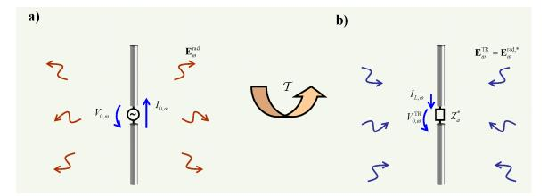
**Figure 2.** (a) An antenna fed by a time-harmonic generator radiates in free-space. (b) Time-reversed problem wherein all the radiated energy returns to the antenna. The antenna terminals are connected to a matched load.
