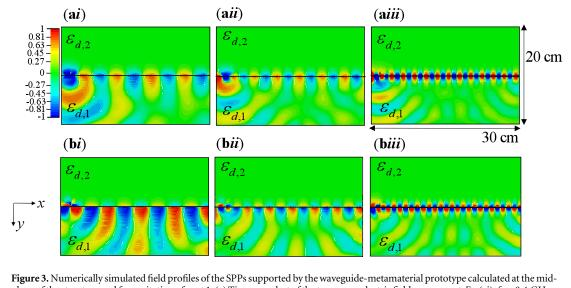
Figure 3. Numerically simulated held profiles of the SPPs supported by the waveguide-metamaterial prototype calculated at the midplane of the structure and for excitation of port 1. (a) Time snapshot of the transverse electric field component  $E_x$ . (ai) f = 8.4 GHz (aii) f = 8.7 GHz (aiii) f = 8.9 GHz. (b) Similar to (a) but for the normal electric field component  $E_y$ .
