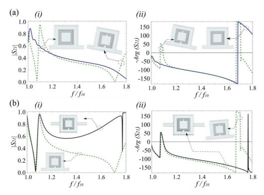
FIG. 6. (Color online) Amplitude (i) and phase (ii) of the transmission coefficient ( $S_{21}$ ) as a function of the frequency. (a) Effect of closing the SRR gap. (b) Effect of centering the input and output waveguides. The dashed (green) curves are the same as in Fig. 4.
