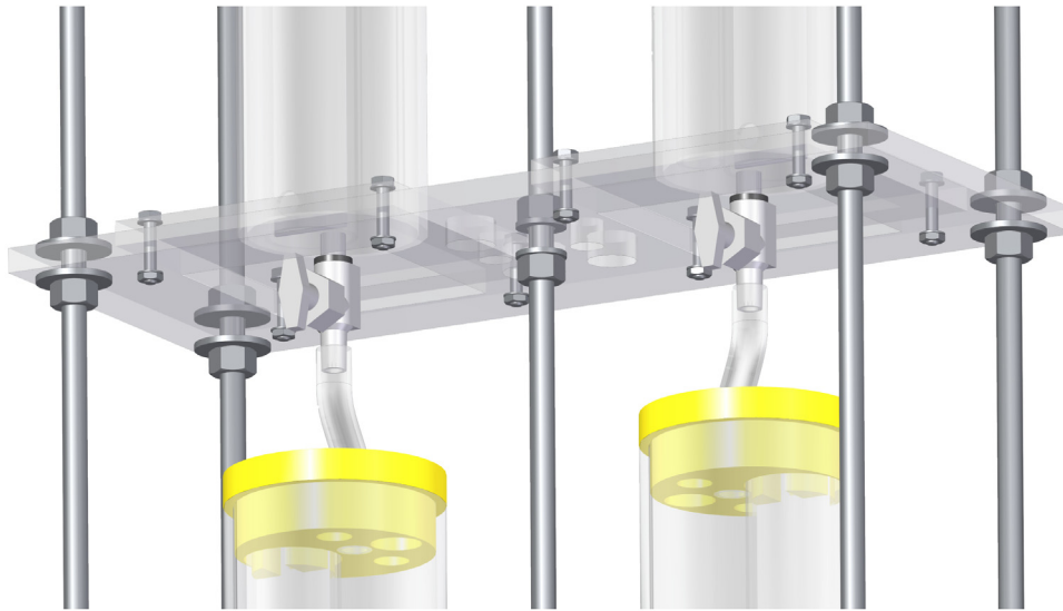
Fig. 3. Coupling of the outlet valves of the upper tanks to the setup.
