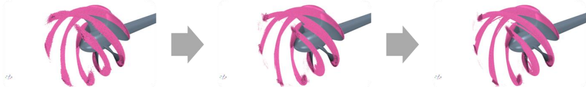
Fig. 5: Tangential vorticity volumetric threshold refinements for iterations two, four and six. Cell sizes are D_{\text{Prop}}/320 , D_{\text{Prop}}/640 and D_{\text{Prop}}/960 , respectively.
