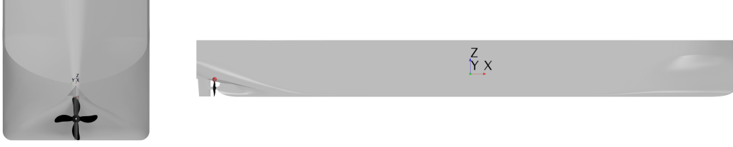
Fig. 1: LDP vessel geometry, point probe and ship-fixed coordinate system at COG.
