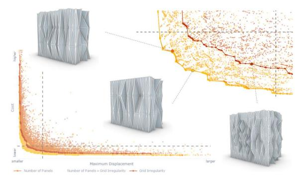
Figure 8.10. Comparison of the previous truss optimizations (orange and yellow) with one with the number of panels fixed at its original value (red).
