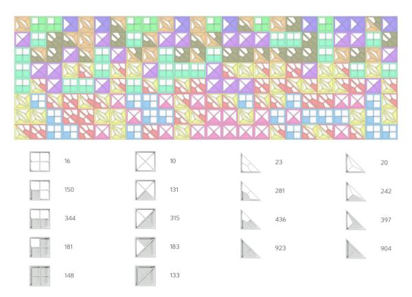
Figure 8.34. Part of the facade 3D model with each type of brick identified with a different color (top) and their frequency of use (bottom).
