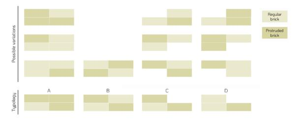
Figure 8.23. Four typologies (A to D) with the corresponding variations resulting from their rotation.
