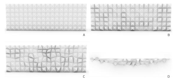
Figure 8.38. Design evolution: creation of squared-based pyramidal elements with (A) equal and (B) random heights, followed by the (C) random deformation of their bases and (D) their distribution on a convex surface together with their heights varying in both directions.
