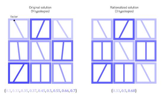
Figure 7.71. Conceptual representation of the rationalization process: on the left, the original solution composed of 9 different elements resulting from the set of factors below; on the right, the solution after the rationalization process with  $n_{typologies} = 3$ , the initial set of nine factors being reduced to three.
