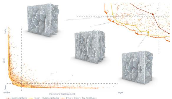
Figure 8.8. Truss optimization with the previous variables plus additional variables for different inner, outer, and top amplitudes of the crystal-like effect.
