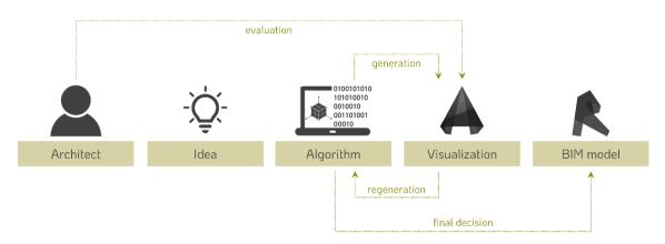
Figure 8.27 AD workflow: the architect presents the design idea to be implemented and, after visualizing the results in the CAD tool, suggests design improvements; this process is repeated until the architect is satisfied with the result, at which point we use the same algorithm to generate its BIM model with the correct BIM families and information.
