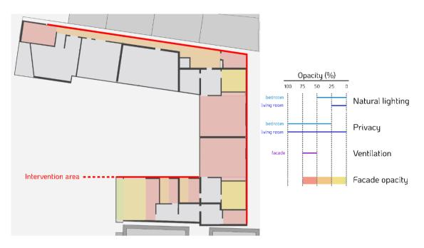
Figure 8.32. On the left: application study plan with red lines representing the facade intervention and colored areas identifying each inside space opacity level; on the right: legend of the different opacity levels with the corresponding daylight, privacy, and ventilation levels.
