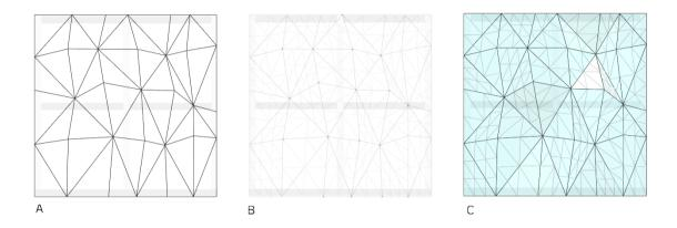
Figure 8.4. Design intent implementation: creating the truss bars (A), horizontal supports (B), and panels (C).
