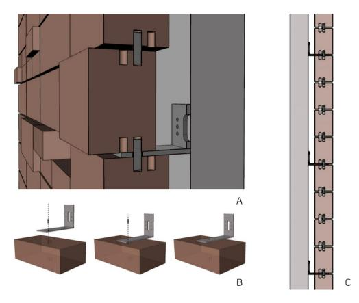
Figure 8.25. Bricks supporting system: A. facade section illustrating the two possible stacking positions; B. angled brackets and metal profiles fitting process; C. facade section showing the thermal isolation zone.
