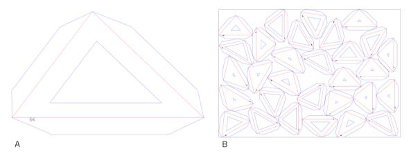
Figure 8.44. A. Triangular panel labelling; B. Nesting of the triangular panels' unfolded drawings.
