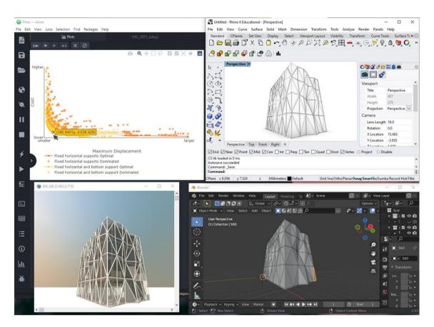
Figure 8.12. Visualization of the solution selected in the interactive graph (top-left) in multiple tools: a point-andclick in one of its dots triggers the generation of the corresponding 3D model in, for instance, Rhinoceros 3D (top-right), POVRay (bottom-left), or Blender (bottom-right).
