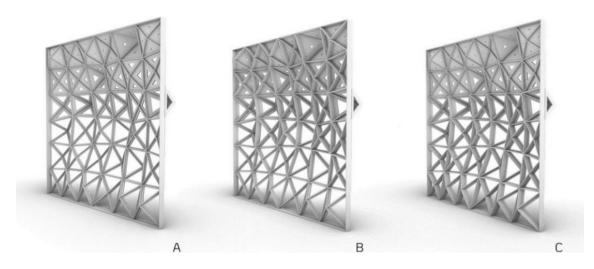
Figure 8.46. Prototype interior view: panels with folded ends with (A) fixed sizes or with their size (B) inversely proportional or (C) directly proportional to the panels' hole.
