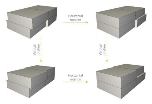
Figure 8.22. Possible rotations of a brick typology.
