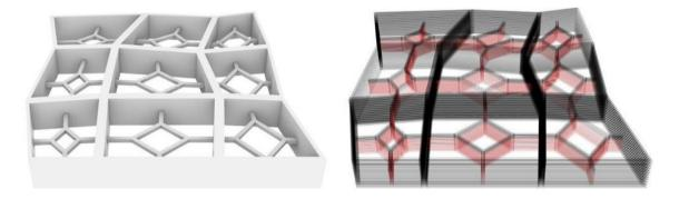
Figure 7.77. The original geometric model and the resulting printing paths (black lines) and support structures (red lines).
