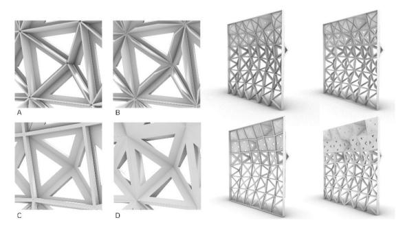
Figure 8.47. Algorithmic exploration of different construction schemes: A. triangular panels with rectangular folds; B. triangular panels with trapezoidal folds; C. pyramidal folded panels with U-profiles hiding their connections; D. three-dimensional triangular panels. On the left, their close-up view and, on the right, the resulting prototype interior view.
