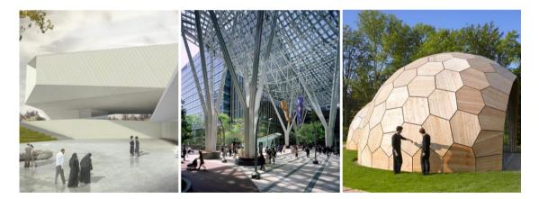
Figure 6.17. Quadrangular and hexagonal paneling examples (from left to right): Museum of Tolerance Jerusalem by Chyutin Architects (©ChyutinArchitects); Tokyo Midtown Plaza roof by Buro Happold, 2005 (©SOM); the Landesgartenschau Exhibition Hall by ICD/ITKE/IIGS University of Stuttgart, 2014 (©Roland Halbe).
