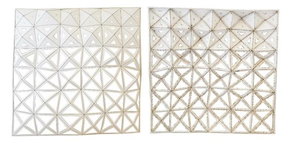
Figure 8.45. Facade panel scaled prototype: outside (left) and inside (right) views.
