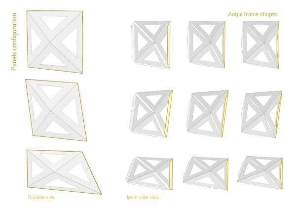
Figure 8.41. Construction details: on the left, two panel configurations and, on the right, their extension with folded ends of varying sizes and shapes.
