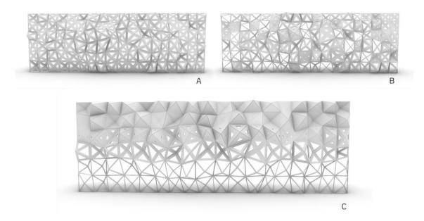
Figure 8.39. Performance-related design variables: obtaining different permeability levels through the creation of panel holes with (A) fixed, (B) random, and (C) gradually changing sizes.
