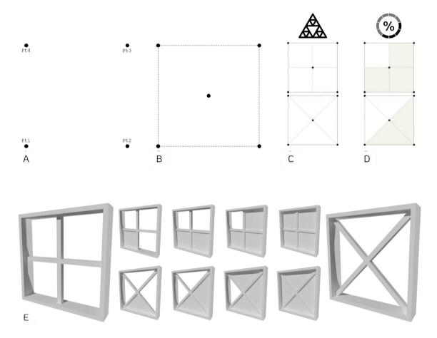
Figure 8.29. Top. the implemented geometric rule: when receiving a set of four points defining the brick's vertices (A), it creates the brick frame and calculates its center (B), while allowing for the selection between two possible rules (C) and different opacity levels (D). Bottom. the range of possible solutions for a given set of four points (E).
