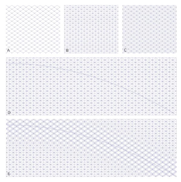
Figure 7.72. Pattern's geometric implementation: creating a rhombus grid (A); mapping the pyramidal elements (B); creating the pyramids' openings (C) while controlling their aperture factor according to their distance to a curve (D-E).
