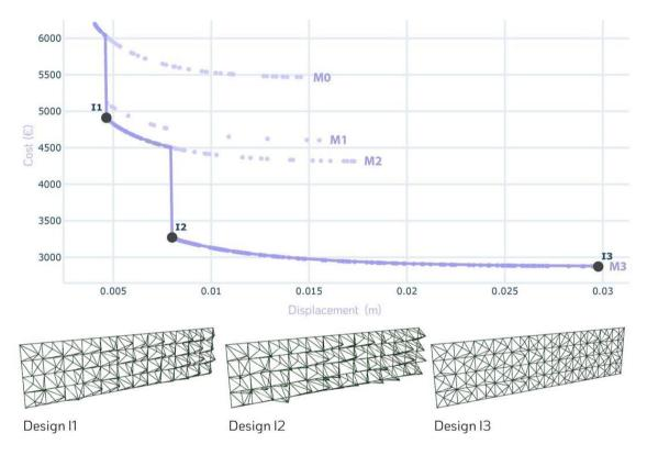
Figure 7.69. Optimization of the truss' structural performance and cost using four materials (M0,M1,M2,M3): on top, the resulting Pareto front (lilac curve) and, at the bottom, three optimal designs (I1, I2, I3).
