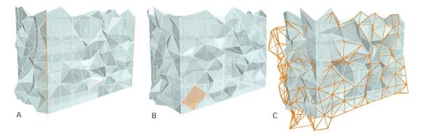
Figure 8.5. Iterative structural analysis using default truss bar materials and cross-sections and gravitational loads automatically calculated from the truss self-weight: A. overlapping truss elements and insufficient physical connections; B. node coplanarities; C. truss deformation tendency. At each iteration, the design was changed according to the results and reanalyzed to check if all problems were solved.
