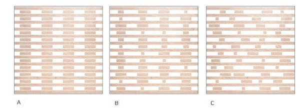
Figure 8.14. Facade panels' geometric evolution: alternating between one full-length bar and a set of equally distanced smaller bars (A); and randomly controlling the smaller bars' size (B) and position (C).
