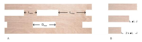
Figure 8.15. Additional geometric restrictions: A. maximum and minimum possible lengths and maximum distance between smaller bars; B. smaller bars' size increment.
