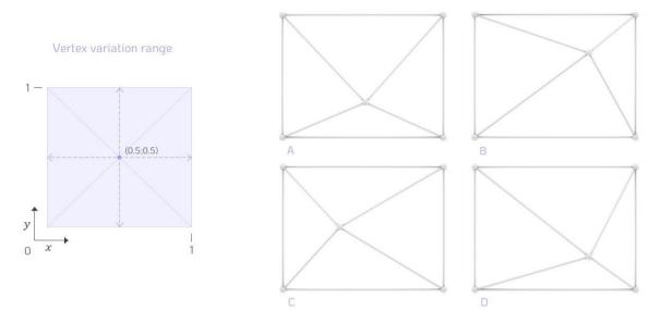
Figure 7.67. Left: ranges between which the pyramids' apices can vary in both x and y directions (e.g., when kx = ky = 0.5 the apex is centered); Right: four pyramids resulting from different factors (A: kx = 0.5; ky = 0.3; B: kx = ky = 0.65; C: kx = 0.35; ky = 0.5; D: kx = 0.7; ky = 0.3).
