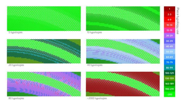
Figure 7.74. Visualization of the typologies' frequency of use for different rationalization levels using a color scheme.
