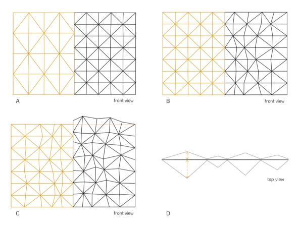
Figure 8.6. Decision variables: A. number of triangular panels; B. grid irregularity; C. top amplitude; D. inner and outer amplitudes.
