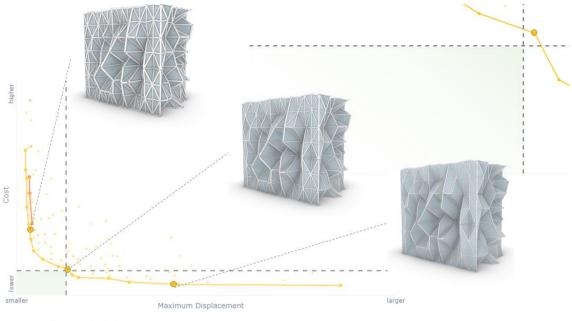
Figure 8.7. Truss optimization with fixed horizontal supports and different truss bar materials and section sizes: bottom left, the area of acceptable solutions identified in green, the horizontal and vertical dashed lines delimit the maximum acceptable cost and displacement, respectively; top right, a close-up view of the acceptable area.
