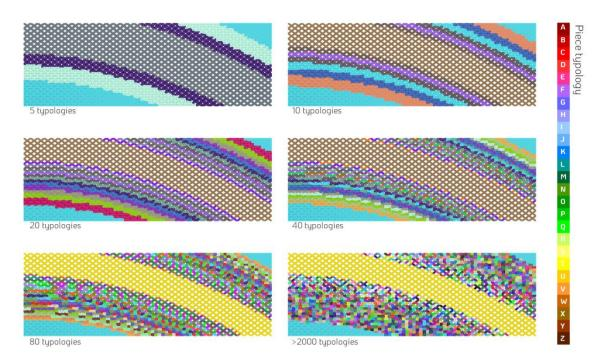
Figure 7.73. Representation of the existing typologies for different rationalization levels using a color scheme.
