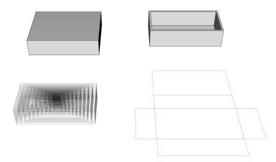
Figure 7.76. Automatic production of technical documentation for different manufacturing techniques: 3D printing, sectioning, laser cutting, and casting.
