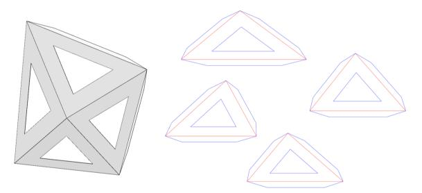
Figure 8.43. Pyramidal element 3D model (left) and corresponding unfolded technical drawings (right).
