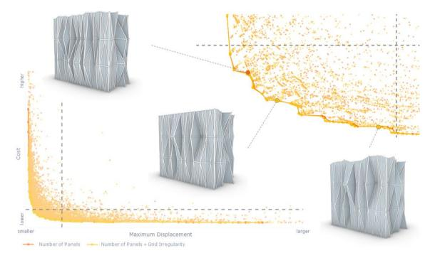
Figure 8.9. Truss optimization with the previous variables plus a different number of panels (orange) and grid irregularities (yellow).
