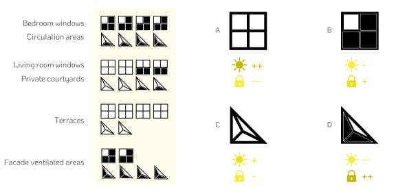
Figure 8.33. Left: the ratios of squared- to triangular-shaped elements of each interior space function; Right: each type of brick privacy (lock symbol) and daylight illumination (sun symbol) levels, with type A corresponding to the highest daylight and lowest privacy levels, types B and C to intermediate levels, and type D corresponding to the opposite.
