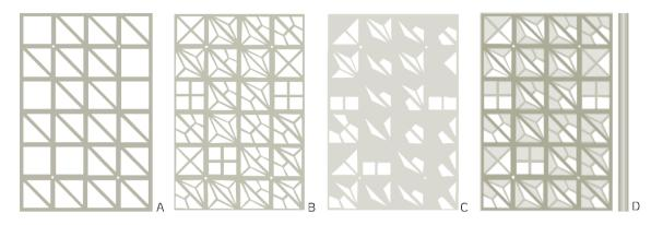
Figure 8.35. A. the outer layers of a wood panel delineating the *cobogó* elements' frame shape; B. its middle layers outlining the *cobogó* elements' interior elements; C. its inner layer producing both the existing voids and opaque areas; D. the resulting wood panel after overlapping the previous layers in a A-B-C-B-A order (front and side views).
