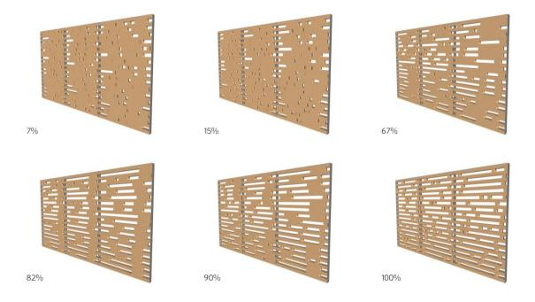
Figure 8.16. Six facade panel configurations with the corresponding sUDI levels.
