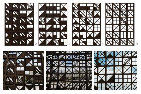
Figure 8.36. Prototypes with different opacities: on top, four typologies with decreasing opacity levels (A to D); at the bottom, three pictures of the produced prototypes.
