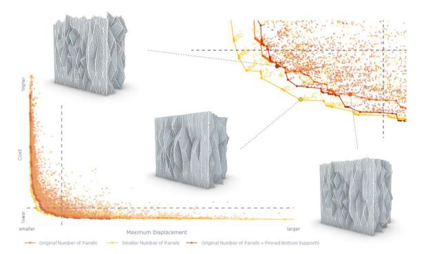
Figure 8.11. Truss optimizations with the number of panels fixed at its original value (orange), at a slightly value (yellow), and at its original value plus the bottom supports pinned (red).
