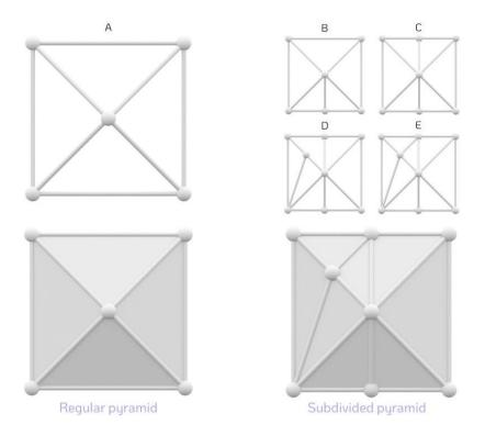
Figure 7.66. Pyramidal truss elements before (A) and after the application of a subdivision rule (B-E).
