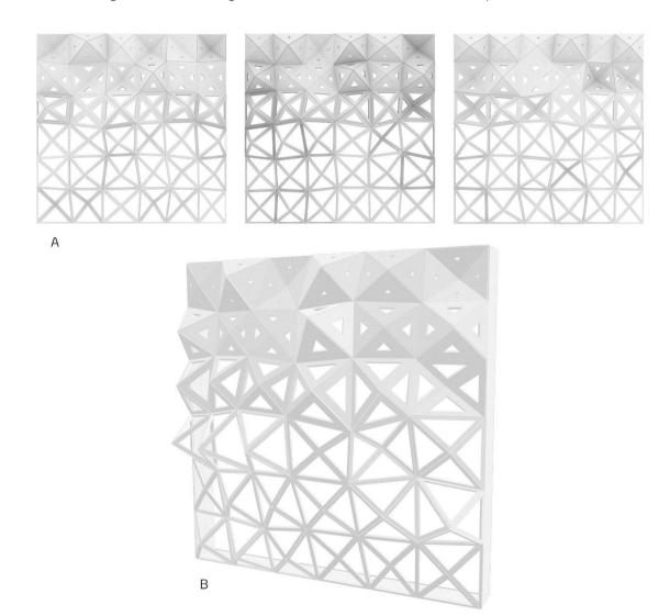
Figure 8.42. The division of the solution into equally sized parts (A) and the creation of an outer frame increasing their structural stability and facilitating their fixation to the building structure (B).
