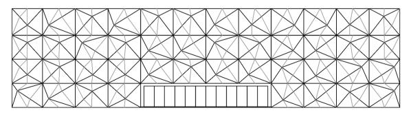
Figure 7.65. Front view of a truss-like facade: the black lines represent the pyramidal truss elements and the grey lines the elements subdividing their faces.
