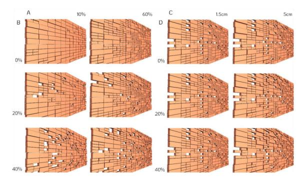
Figure 8.21. Design variations explored: A - Percentage of four small bricks; B - Percentage of absent bricks; C - Protrusions' depth size; D - Percentage of protruded bricks.
