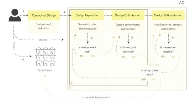
Figure 8.1. AD workflow: design intent definition (1) and implementation using the framework (2); design geometric exploration (3) and improvement regarding a certain fitness criterion (4); control of the design's manufacturing cost and waste (5) and selection of the final solution (6); A. iterative process of geometrically adjusting the design to meet the fitness goal(s) set; B. iterative process of balancing design intent, performance, and feasibility.
