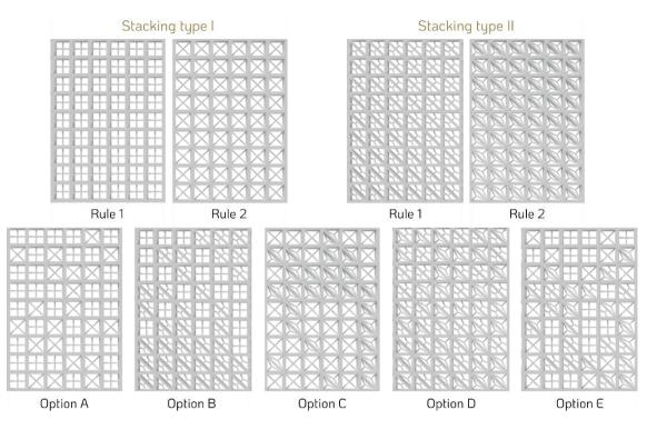
Figure 8.31. Pattern evolution: On top, two stacking types using rule 1 and rule 2; on the bottom, different options explored using both rules and the stacking type I (A), rule 1 and both stacking types (B), rule 2 and both stacking types (C), both rules and the stacking type II (D), and all rules and stacking types (E).
