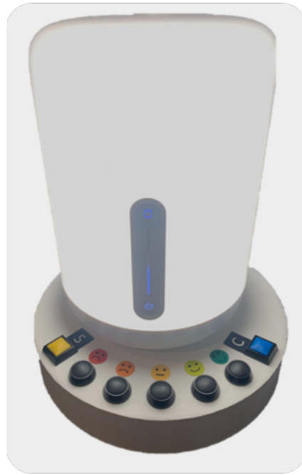
Fig. 1. The Emotions2Us prototype consists of a smart lamp and a seven-button keyboard.
