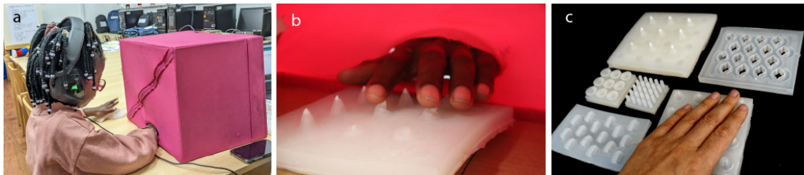
Fig. 2. a) A child interacting with shape-changing skin inside the pink box during the study; b) captures the internal view of touching the spikes skin; c) a collection of shape-changing skin samples that change users' haptic experiences through pneumatic control.
