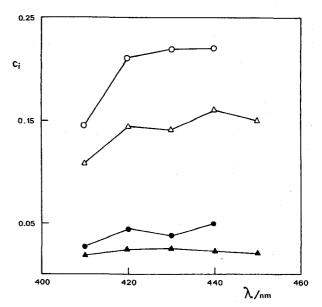
FIG. 4. Decay parameters vs emission wavelength. ( $\triangle$ ) C<sub>1</sub>, [DPA] =  $1.0 \times 10^{-3}$  M; ( $\triangle$ ) C<sub>2</sub>, [DPA] =  $1.0 \times 10^{-3}$  M; ( $\bigcirc$ ) C<sub>1</sub>, [DPA] =  $1.0 \times 10^{-2}$  M; ( $\bigcirc$ ) C<sub>2</sub>, [DPA] =  $1.0 \times 10^{-2}$  M.
