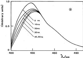
FIG. 5. Time resolved fluorescence spectra of DPA solutions. (a)  $[DPA] = 5.0 \times 10^{-2} \text{ M}$ ; (b)  $[DPA] = 1.0 \times 10^{-3} \text{ M}$ .
