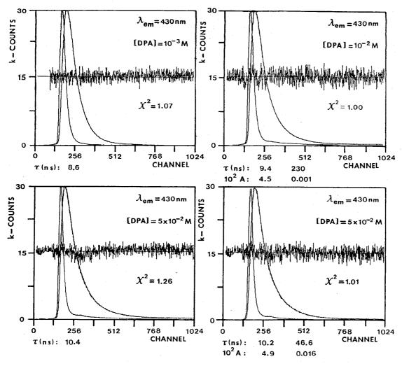
FIG. 2. Fluorescence decay curves of DPA solutions analyzed with a sum of exponentials.
