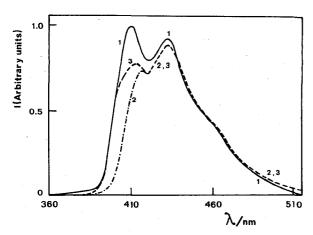
FIG. 1. Fluorescence spectra of DPA in benzene. (1) [DPA] =  $1.0 \times 10^{-6}$  M; (2) [DPA] =  $5.0 \times 10^{-2}$  M; (3) Curve 2 corrected for reabsorption using Eq. (15).
